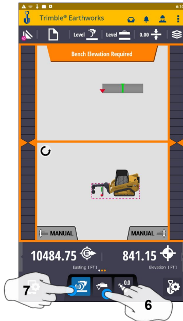
6. Select Blade Tip Focus Point 7. Place Blade Tip at Elevation and Touch Bench
