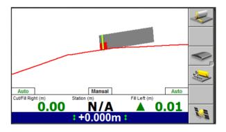
One Point Focus is used for narrow surfaces such as shoulders or slopes.
