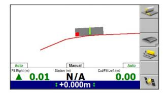
One Point Center is the default setting used for long or wide surfaces. It also allows for shaping crowns by holding the slope past the crown-point.
