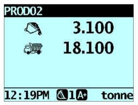
Roll the bucket partially forward, tipping product into the truck. The Indicator will give a live weight as it is tipped into the truck.
