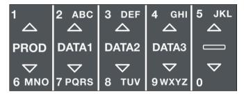
Data field values can be selected before starting a new load. The following example assumes that **Data 1** has been configured to hold customer names and shows how to select a customer name to record against the weighing data.
