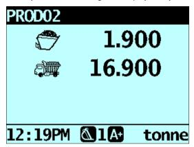
Roll the bucket partially forward, dumping the product. The Indicator will display the weight in the bucket and the potential weight of the truck.
