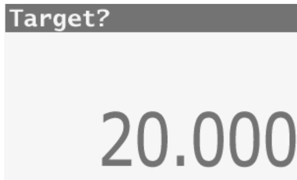
3. Use the numeric keys to enter the new target. Press Enter to accept.
