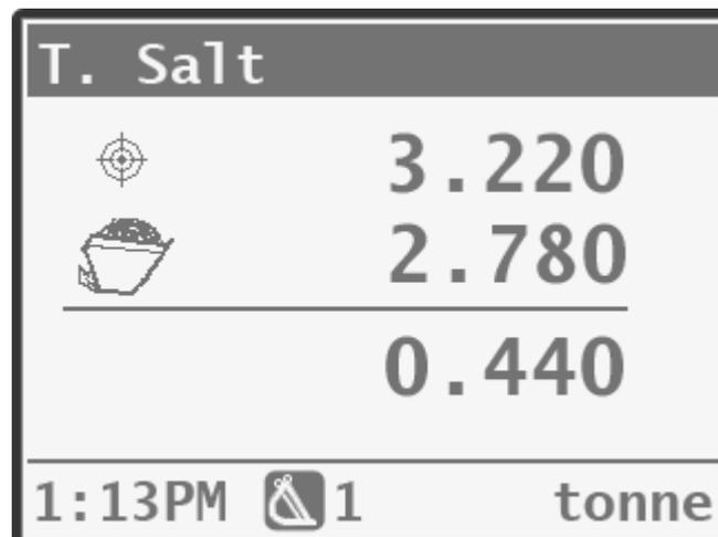
6. As the truck is loaded the target amount will decrease. The aim is to get as close to zero as possible. A positive to load value is under the target, a negative to load value is over the target.
