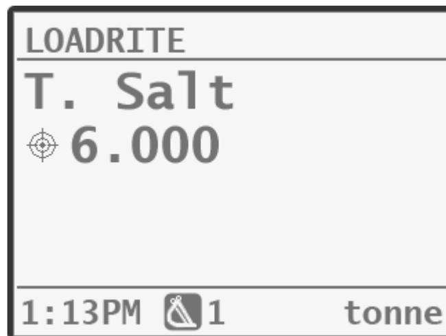
5. As the weight is lifted the target weight is displayed along with the current lifted weight and the potential weight if the lift is loaded.
