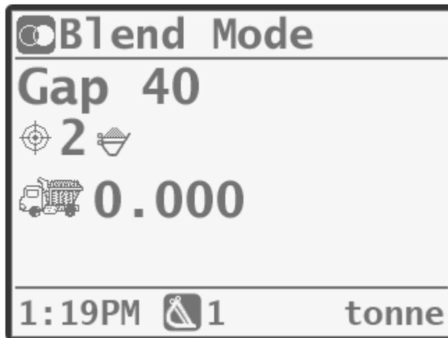
3. Lift and add the load as normal. The screen will count down the number of loads to be lifted.
