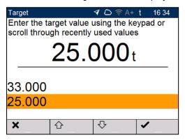
3. Use the keypad to enter the target weight value , or use  $2^{10}$  and  $2^{10}$  to select a previous target weight value, if available.
