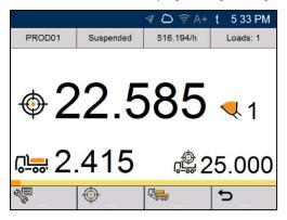
Raise a bucketload of product through the Weighing Zone using constant engine revs. The Green light will flash during the lift. If Weight Preview functionality is enabled, a preview of the weight will display during the lift:
