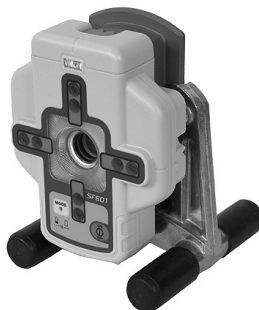
SF601 attached to the optional pipe laser target base
