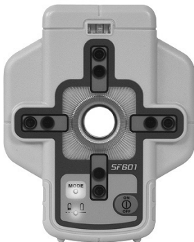
SF601 attached to the optional pipe laser target base
